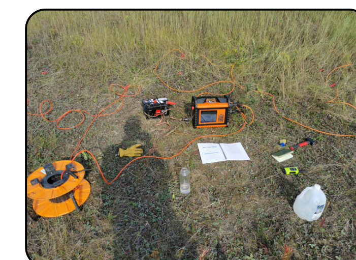
Figure 5: ABEM Terrameter LS 2 during data collection.
