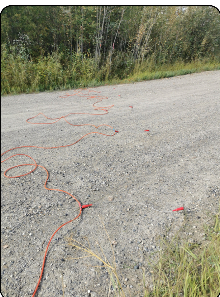
Figure 4: ERT survey line crossing a road.
