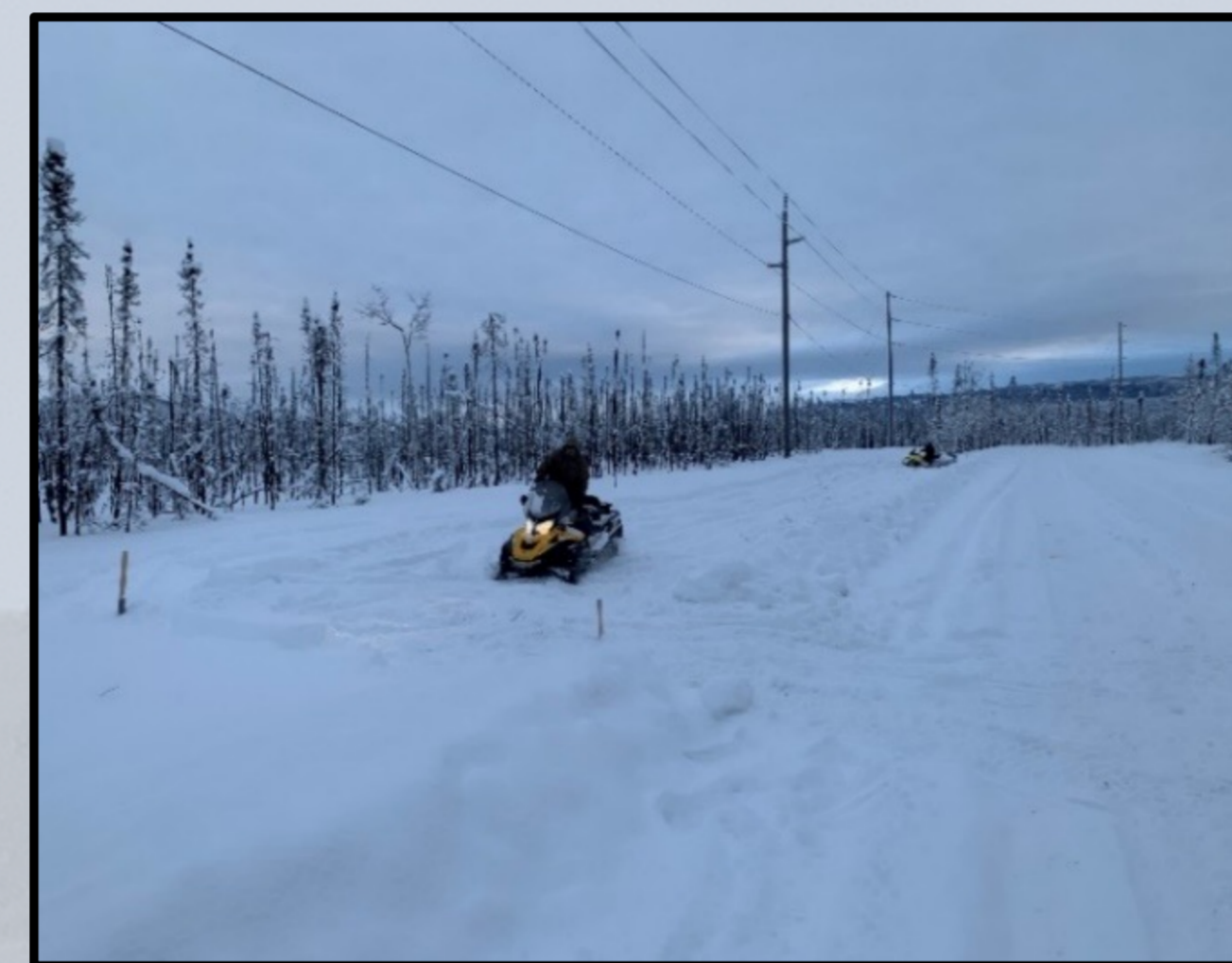
Figure 3: Compaction of the snowpack at the M2 field site on November 29th, 2020.
