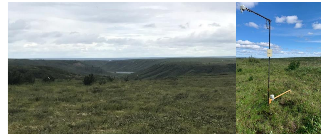
Figure 2. (Left) Area with high variability in topographic slope. (Right) Inclinometer and snow depth sensor at one of the six sites.
