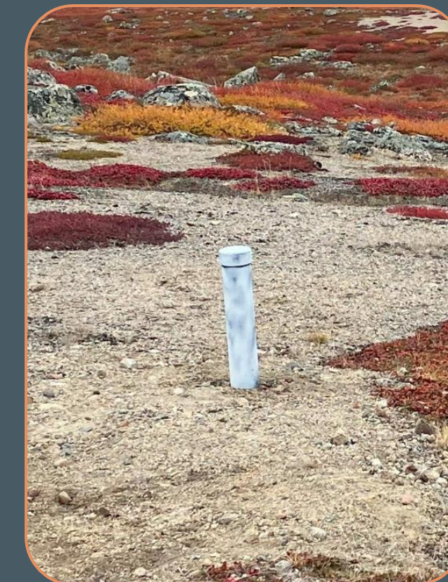
Figure 2. A borehole drilled and anchored into the permafrost. Installing temperature sensors at defined intervals allows for ground temperature to be recorded over many years and permafrost change to be tracked.
