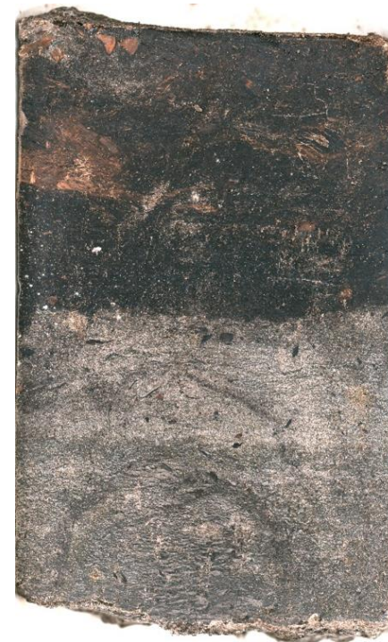
Sharp transition between ice-rich sandy silty peat and inorganic ice-poor silts
