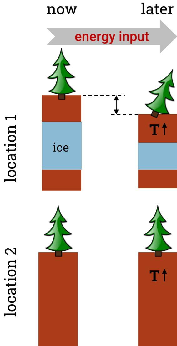
Permafrost can turn energy input into hazards via temperature increase and ground-ice loss
